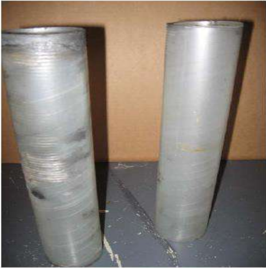
Damage to mylar sleeves, typical through out.
