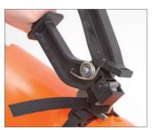
STEP 2: Trim off excess band using cutting blade.\*
