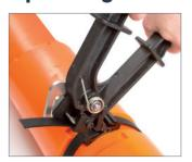
STEP 1: After hand tightening the band and buckle assembly, pass the tool over the excess and locate against the buckle. Squeeze handles together to tighten further.\*
