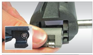
NOTE – Take care to note the orientation of the spring for reinsertion
