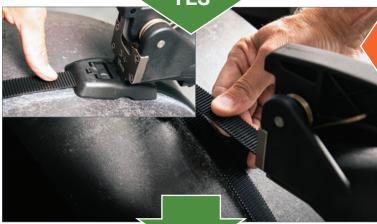
NOTE – The Mountz torque wrench is factory set to the correct torque requirement for the specified product being used. The set torque is marked on the wrench.
