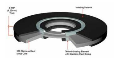
The DEFENDER™ sealing/isolating gasket system is designed for critical/extreme applications. Manufactured with a 316 stainless steel core retainer and laminated on both sides with high strength laminates, the DEFENDER™ gasket is resistant to deforming under load and is used when electrical isolation and corrosion control are required on pipes containing gas,
